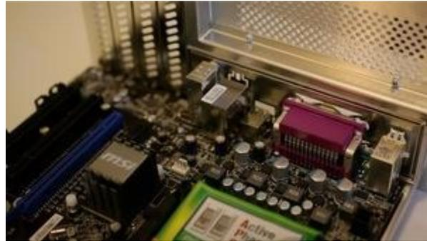
Open up your motherboard box and take out the I/O shield, which is the metal plate that protects the ports on the back of your motherboard. You should see a rectangular space in the back of your case where this should go. Snap it into place. This takes quite a bit of force, so make sure all four sides are snapped in securely.
