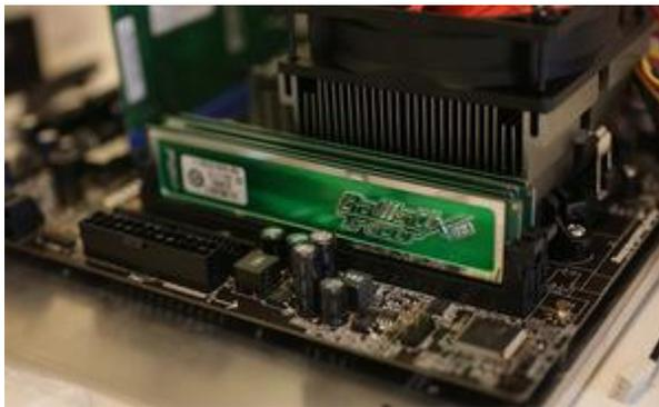
Installing RAM is very simple. Find the RAM sockets on your motherboard, and pull the two clips on the side down. Line up the notch in your RAM stick with the notch in the socket, and press the RAM down into place. This might take a bit of pressure, so don't worry about being overly gentle. The clips should snap back into place when the RAM is fully in the socket.
