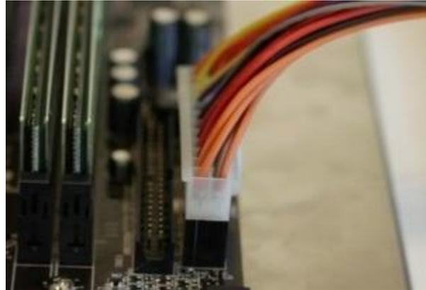
**A 4-pin Motherboard Cable:** You should also have a separate 4-pin cable coming out of your power supply, and a small 4-pin socket somewhere else on the motherboard. This plugs in the same way as the 24-pin cable—just push down until it locks into place.
