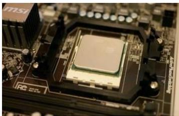
Open up your processor's box and gently take it out. Your processor is one of the more fragile parts of the build, so this is one step in which you'll want to be careful. Find the corner of your processor that has a gold arrow on it, then look at your motherboard's processor socket for a similar arrowed corner. Line these two arrows up; this is the direction your processor will go into the socket.
