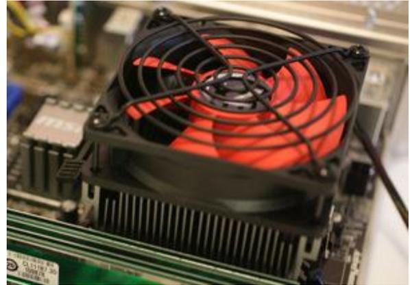
Once your processor's in, grab the cooler that came with your processor (remember, if you got an OEM processor you have to buy a cooler separately). It should already have some silver thermal paste on the bottom. If not, you'll need to pick some up from the computer store and put a very thin line on your processor—I usually use about the size of a grain of rice or two, that's all.
