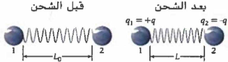
$$F_s = F \Rightarrow k_s \Delta x = \frac{kq_1 q_2}{r^2} \Rightarrow k_s (L_0 - L') = \frac{kq^2}{(L')^2} \Rightarrow q = \sqrt{\frac{k_s (L')^2 (L_0 - L')}{k}}$$
