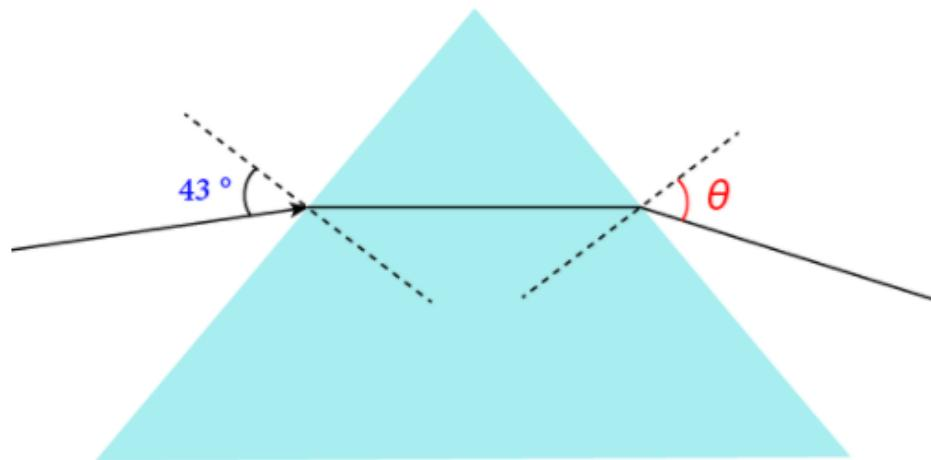
Determine the angle of the exiting light  $\theta$ .
