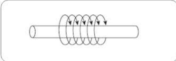
Option D shows a horizontal wire with five concentric circular arrows around the wire, representing the magnetic field lines.
