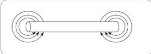
Option B shows a horizontal wire with two sets of concentric circular arrows around the wire, representing the magnetic field lines.
