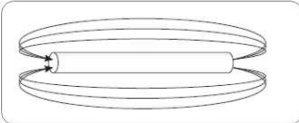
Option C shows a horizontal wire with two sets of concentric elliptical arrows around the wire, representing the magnetic field lines.
