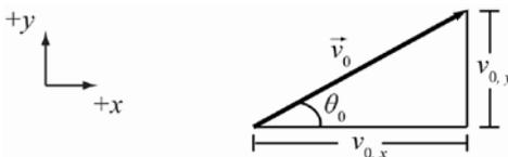
The lengths of the component vectors of  $v_0$  are  $v_{0,x} = v_0 \cos \theta_0$  and  $v_{0,y} = v_0 \sin \theta_0$ . Velocity is a vector quantity, so  $\vec{v} = v_x \hat{x} + v_y \hat{y}$ . Let  $v = |\vec{v}|$ . Then,  $v^2 = v_x^2 + v_y^2$ . The velocity vector  $\vec{v}$  has component vectors  $v_x = v_0 \cos \theta_0$  (horizontal component is constant) and  $v_y = v_0 \sin \theta_0 - gt$  (which changes relative to time).
