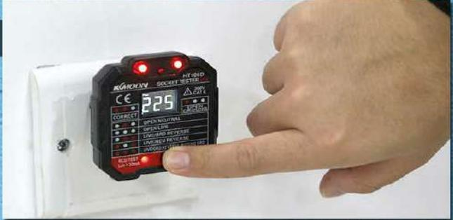
meter can quickly test socket if connects positive and negative pole as request and whether household power protection systems works well or not to ensure the household electrical safety
