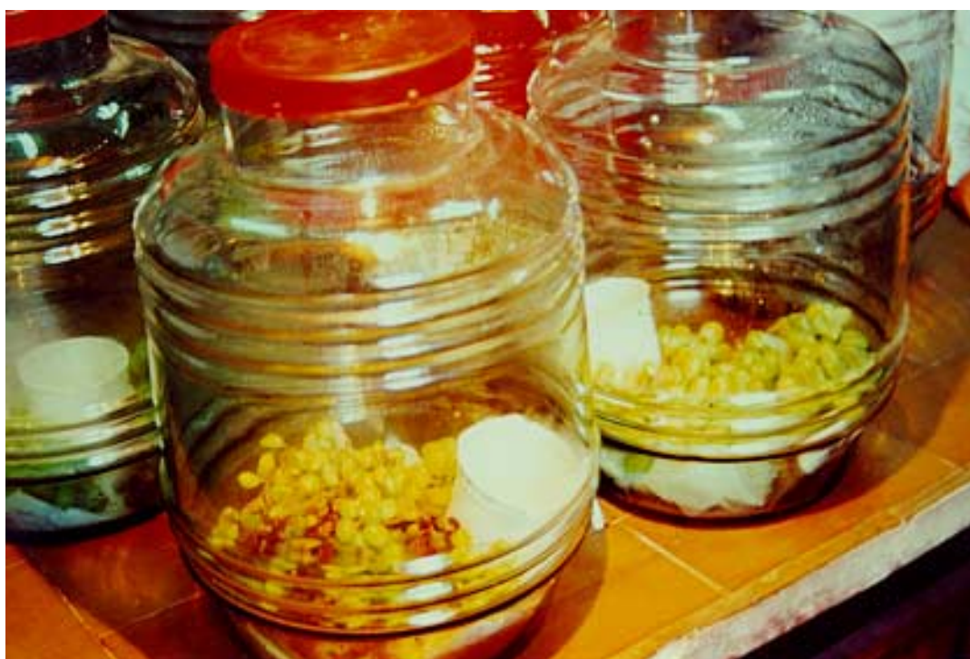
Fig. 24 Flask jars used to provide high humidity conditions for fungus development in grape clusters.
